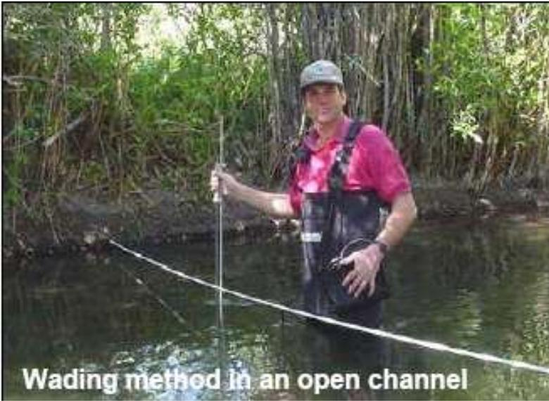
Wading method in an open channel
