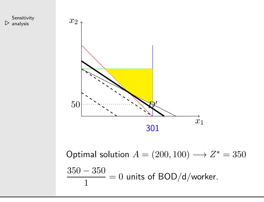
Sensitivity ▷ analysis **Binding constraint** - constraint that is satisfied in the equality by the optimal solution (constraints (2) and (3) in the keeping the river clean problem)
