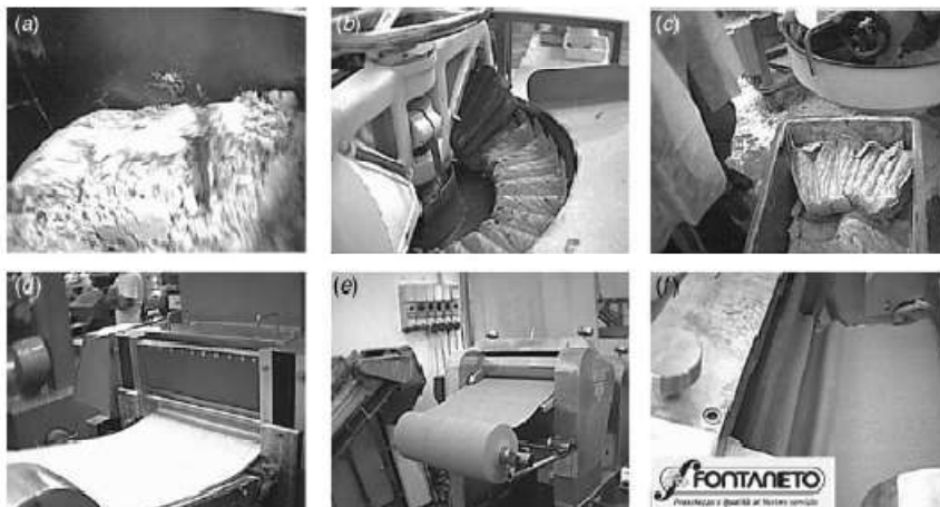
Artisanal fresh pasta-making process: mixing (a); dough kneading with gramola (b); dough cutting (c); intermediate dough sheeting (d); final sheeting (e); pasta after the first pasteurization (f). (Courtesy of Fontaneto, Italy).
