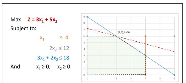
X1 number of window batch; X2 number of glass doors batch Profit of windows batch = 3 profit of doors batch = 5 (K $\in$ )
