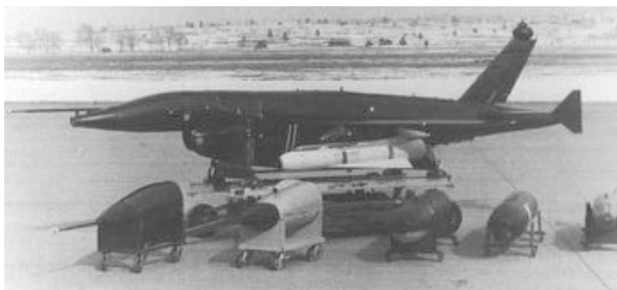
Fig. 4.8 The BGM-34C was another member of the Ryan Model 147 family. It was a multi-role drone capable of performing reconnaissance, electronic countermeasure and strike missions (Photo Credit: US Air Force)
