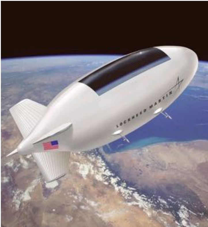
Fig. 4.33 High-Altitude Airship (HAA) developed by Lockheed Martin. It is a solar-powered, untethered, long-endurance, high-altitude demonstrator (Photo Credit: US Missile Defense Agency)
