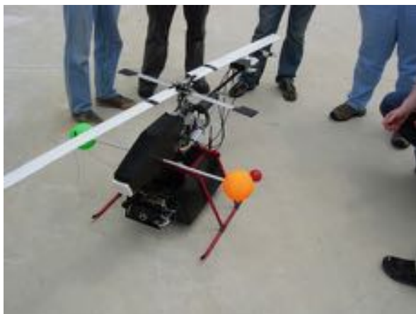
Fig. 112.5 One of the helicopters, Marvin, has attached at its nose a fire detector sensor
