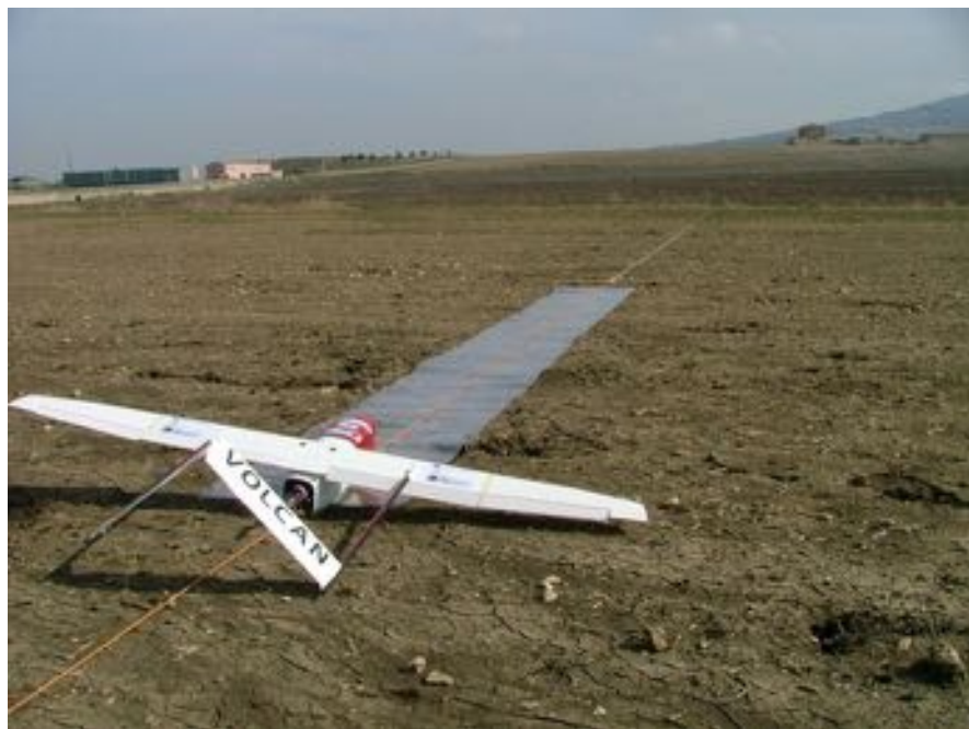
Fig. 111.11 The Volcan UAV ready to be launched by means of an elastic rope
