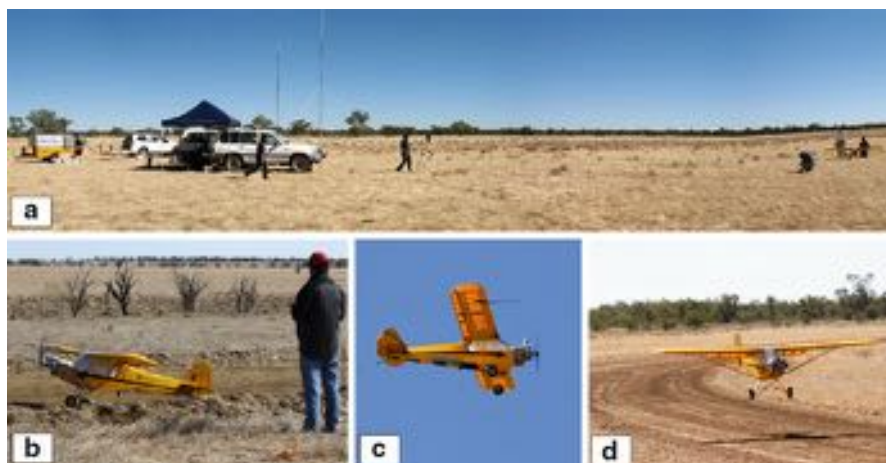
Fig. 116.10 The fixed-wing, 1:3 scale J3 Cup UAV platform used in woody weed and wheel cacti surveillance missions. (a) Typical GCS setup in a remote country site in Northwest Queensland. (b) The UAV taking off, under a human pilot control, from an unsealed road in the bush. (c) The UAV in autonomous flight. (d) The UAV landing onto an unsealed road
