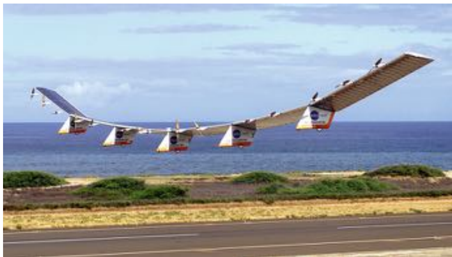
Fig. 4.25 The Helios UAV developed by NASA and AeroVironment. During its second high-altitude flight, it reached 96,863 ft, shattering the existing world altitude record for sustained level flight for both propeller and jet-powered aircraft (Photo Credit: NASA)
