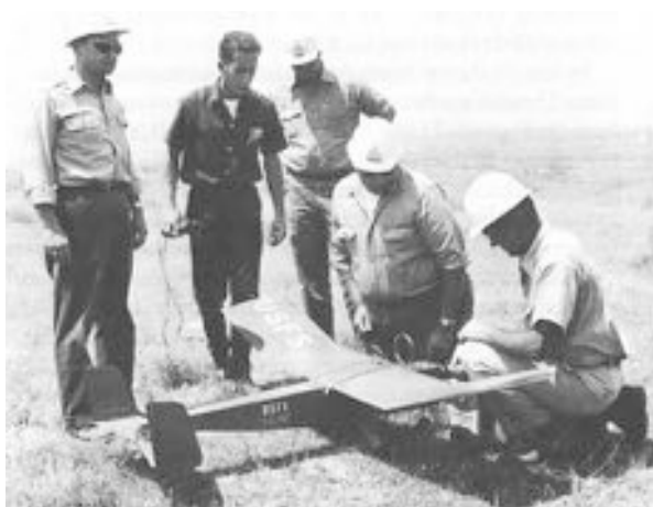
Fig. 113.13 The low-altitude retrievable probe (LARP), a radio-controlled “drone” airplane. The LARP was designed to fly in and around the smoke column of a fire, gathering weather information (From Wilson and Davis 1988)
