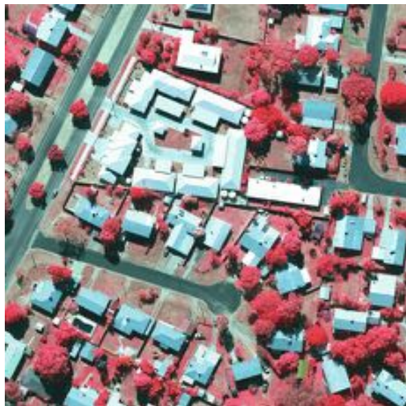
Fig. 20.2 Typical infrared image with 10 cm spatial resolution taken from an aircraft onboard camera (image courtesy of Ergon Energy and the Cooperative Research Centre for Spatial Information (CRCSI))
