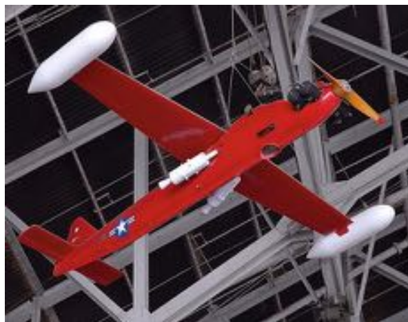
Fig. 4.6 The SD-1, also known as the MQM-57 Falconer, was the first reconnaissance drone of the US Army and remained in service until the 1970s (Photo Credit: National Museum of the USAF)
