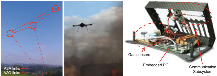
Fig. 33.7 Example experiments carried out in the AirShield project: validation of A2G and A2A links ( left ), validation of sensor data transfer ( middle ), gas sensor and communication payload ( right )
