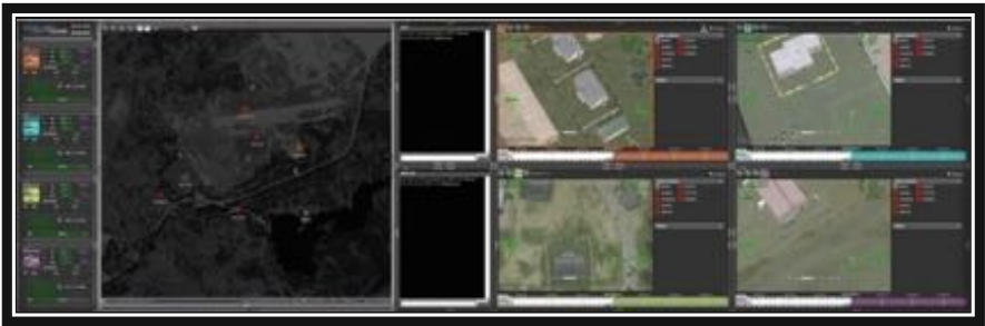
Fig. 101.15 Right monitor shows sensor videos from four UAVs and associated control and DVR tools in a Vigilant Spirit Control Station
