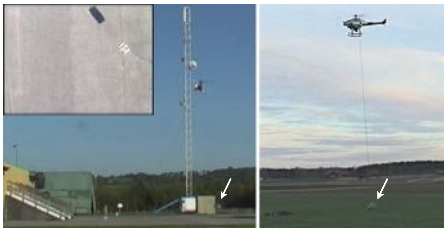
Fig. 37.38 Two frames of video presenting the prototype mechanism for carrying and releasing packages using an electromagnet. An arrow points to a package being carried. The top left picture presents the onboard camera view
