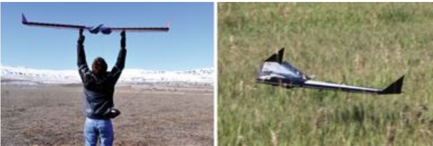
Fig. 117.8 AggieAir bungee launch and skid landing
