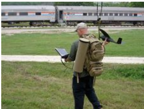
Fig. 4.29 The Nighthawk is the evolution of the BATCAM foldable UAV (Photo Credit: NIST)
