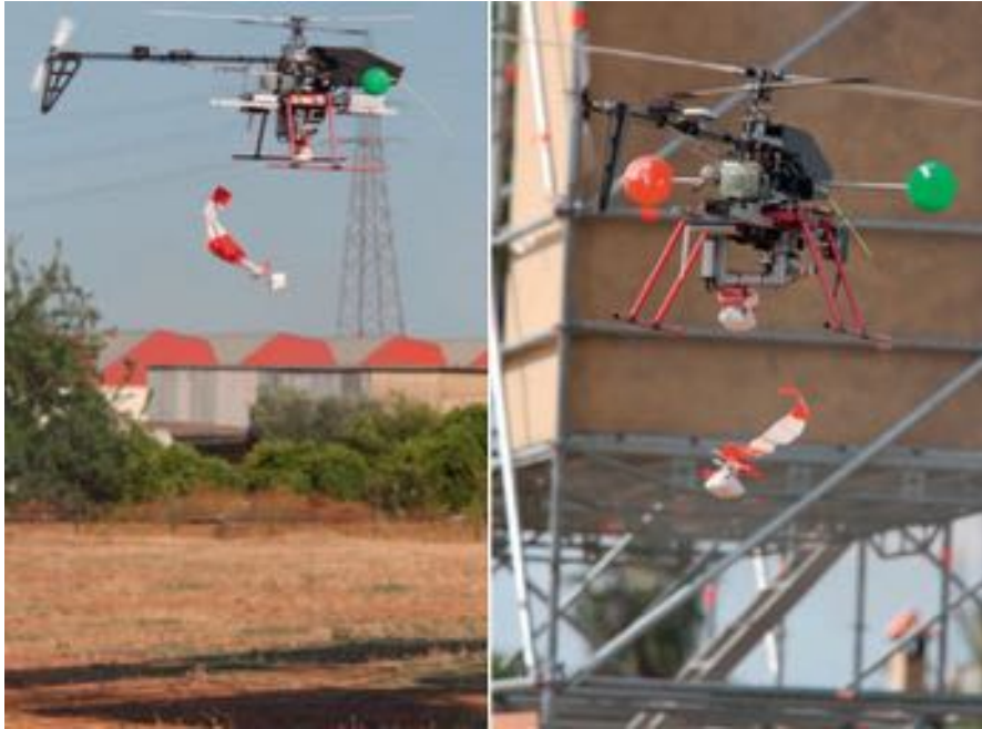
Fig. 112.22 Automatic deployment of WSN nodes using Marvin helicopter UAS
