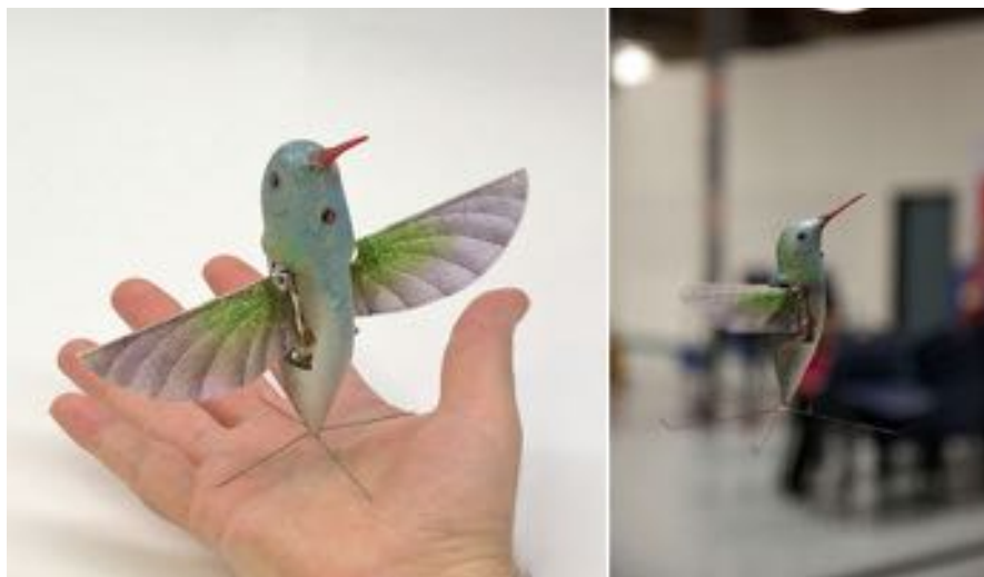
Fig. 56.25 Nano Hummingbird (AeroVironment Inc.) sitting in the palm of a hand and in hovering flight (Photos courtesy of the AeroVironment Corporation)
