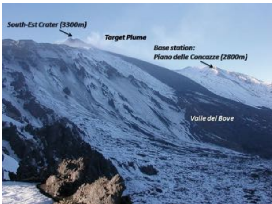
Fig. 111.12 A typical mission of Volcan UAV on the top of Mt. Etna. After takeoff from the base station in Piano delle Concazze, the UAV will reach the target plume and will start to collect samples. Then it will return to the base station to be recovered
