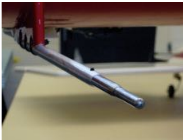
Fig. 18.5 UMN's Thor instrumented with five-hole pitot tube from Goodrich to measure airspeed, \alpha , and \beta
