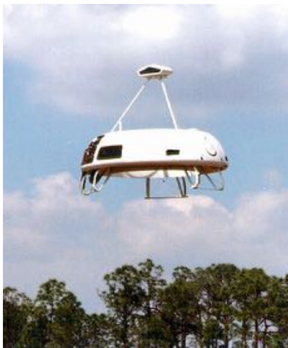
Fig. 4.35 The Sikorsky Cypher uses a shrouded twin-rotor design (Photo Credit: US Navy)
