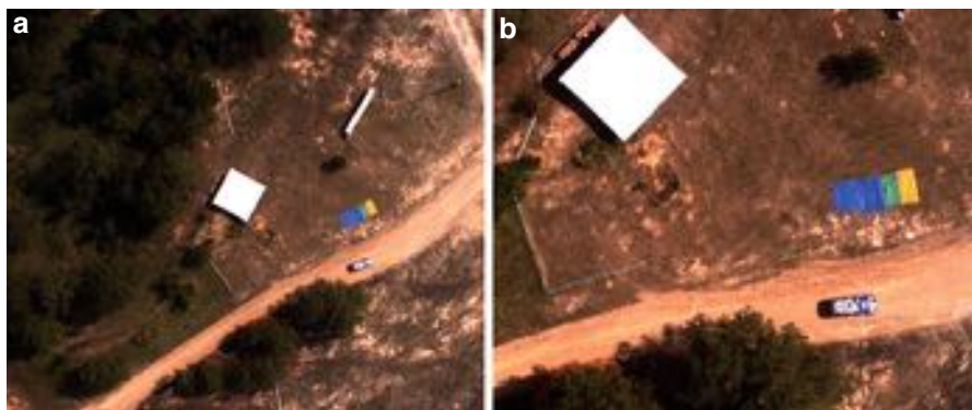
Fig. 71.8 UAV onboard computer vision. The mission processor processes images from the onboard digital camera in real time. The target location is at the colored tarps in the center of the images. The UGV navigated to the target location after the target was detected from the UAV. Images are shown from each of the 2 UAVs, with different camera lenses and flying at different altitudes (a) 8 mm lens at 300 m. (b) 16 mm lens at 250 m
