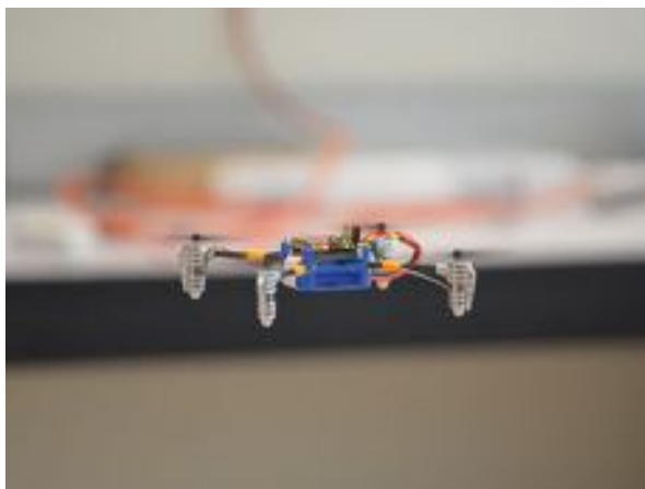
Fig. 11.9 A full working prototype quadrotor MAV, KayLion, designed and built by the National University of Singapore (NUS)
