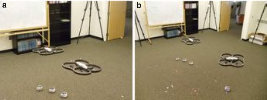
Fig. 84.11 Photos showing the convoy protection and threat neutralization as carried out by the hardware platform. (a) Two UAVs protect the convoy while maintaining spacing from one another. (b) One UAV is dispatched to visit a threat, while the other remains with the convoy
