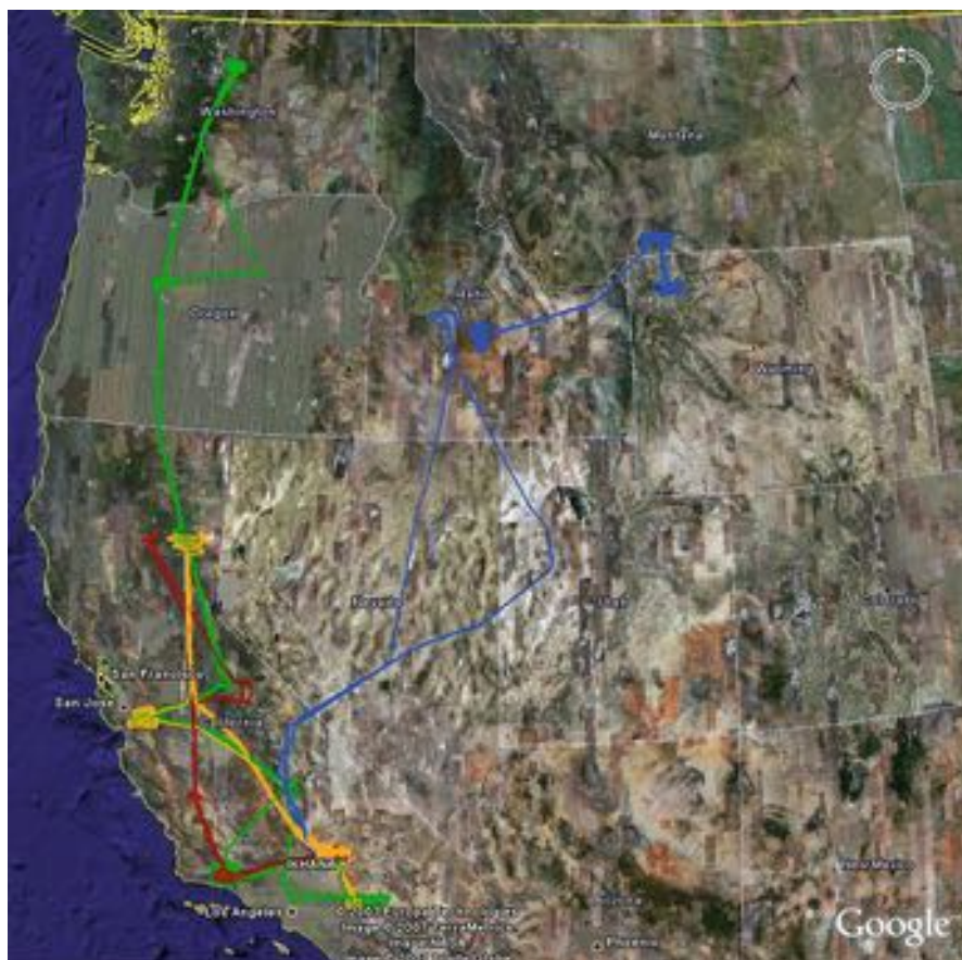
Fig. 113.18 The NASA Ikhana UAS Western States UAS Fire Imaging Mission flight tracks overlain in GoogleEarth. The four missions, spread throughout the summer of 2007, ranged in duration of 9.5–20 h, and covered from 1,400 to 3,200 nmi for each mission
