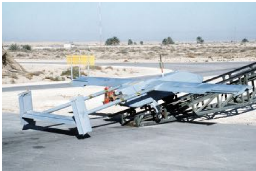
Fig. 4.15 An RQ-2 Pioneer ready for launch during operation Desert Shield (Photo Credit: US Marine Corps)
