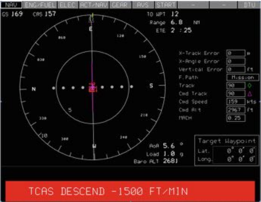
Fig. 77.4 TA/RA/“Clear of conflict” indication (extract from Command and Control HMI)
