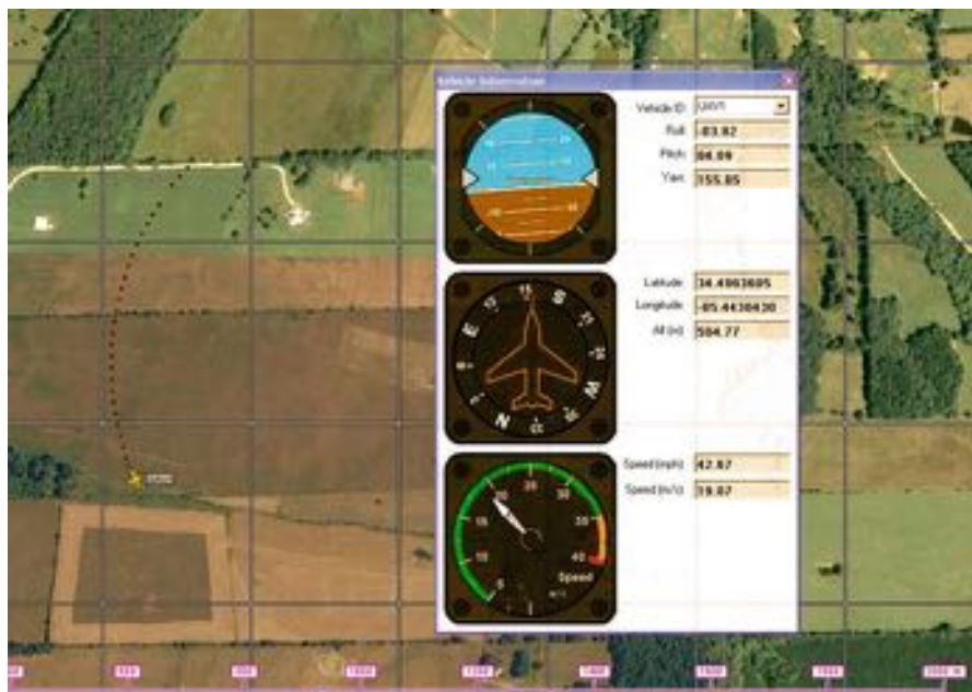
Fig. 71.9 Using the FalconView™-based ground station, multiple UAVs and UGVs can be displayed, with video overlays and system status. The FalconView™ plugin can also send mission-specific commands to the mission processor
