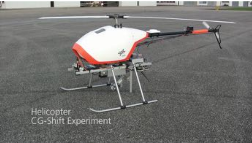
Fig. 114.14 Experimental platform with pendulum for displacement of the helicopter CoG
