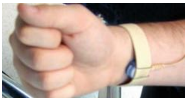
Fig. 101.10 Tactile wrist pads as high priority alert cue
