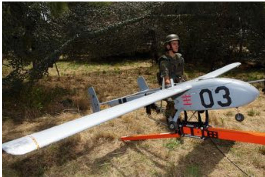
Fig. 105.13 ANTEX-X02 #03 ready for catapult launch
