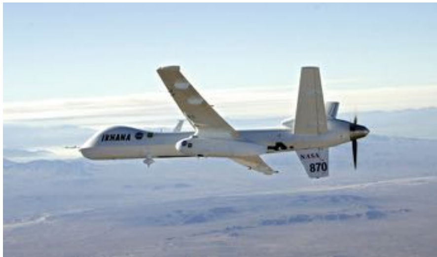
Fig. 4.26 The Ikhana is a Predator B UAV acquired by NASA and retrofitted for Earth science missions (Photo Credit: NASA)
