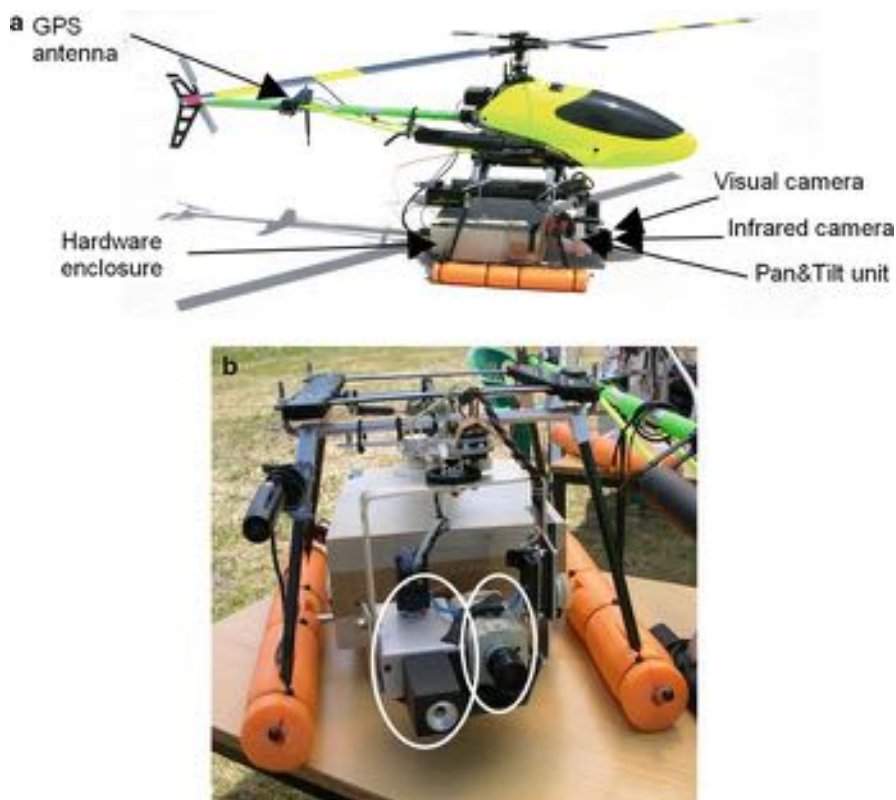
Fig. 112.4 (a) Main sensors and components of Heliv helicopter used in forest fire perception experiments. (b) Detailed picture of the pan and tilt device with one Raytheon 2000AS OEM infrared micro-camera and one visual camera
