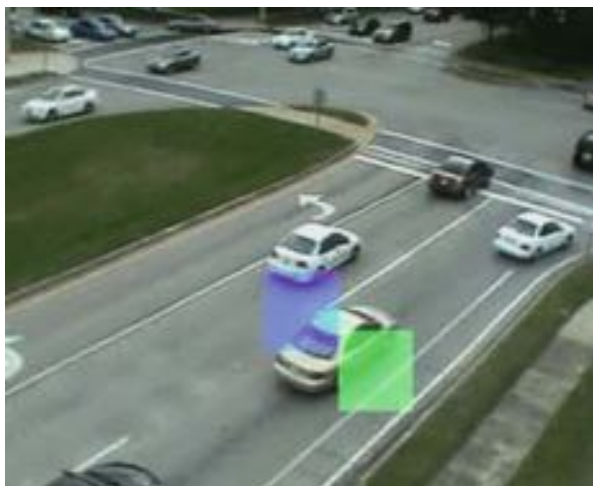
Fig. 110.4 Colored boxes show implementation of virtual detectors in the image processing technique (Puri 2008)
