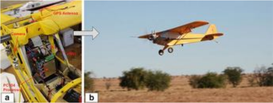
Fig. 116.11 (a) The fixed-wing 1:3 scale J3 Cub UAV platform with the onboard avionics and downward-pointing color camera, (b) The UAV flying over woody weed infestation
