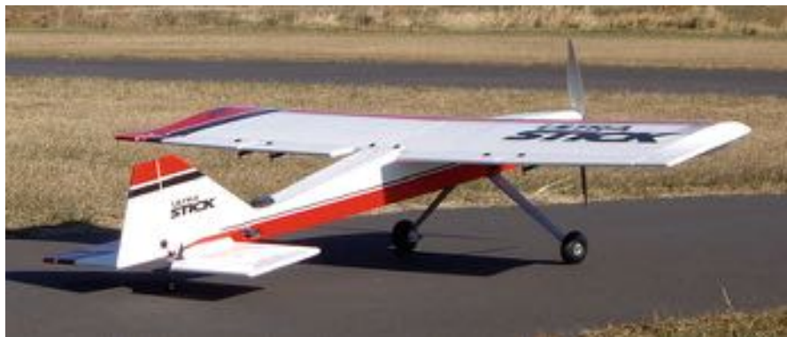
Fig. 18.2 Free-flying for Subscale Experimental Research (FASER) UAV (a modified Ultra-stick 120)
