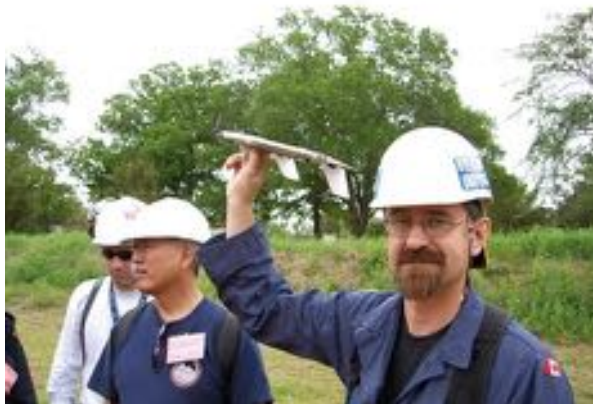
Fig. 4.28 The WASP is a MAV that can carry an EO payload and has an endurance of over 1 h (Photo Credit: NIST)
