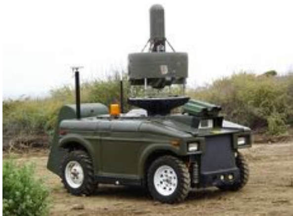
Fig. 4.34 The iSTAR MAV duct-fan aircraft built by Allied Aerospace (Photo Credit: US Navy)
