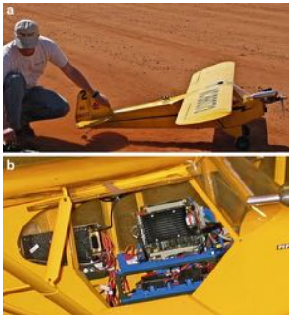
Fig. 71.5 UAV platform. (a) The UAV platform is configurable for different mission requirements, payloads, and sensors. (b) The basic research payload (on the right ) includes a mission processor, datalink, and digital camera. The mission processor connects to the autopilot (small box on the left ) over the serial port
