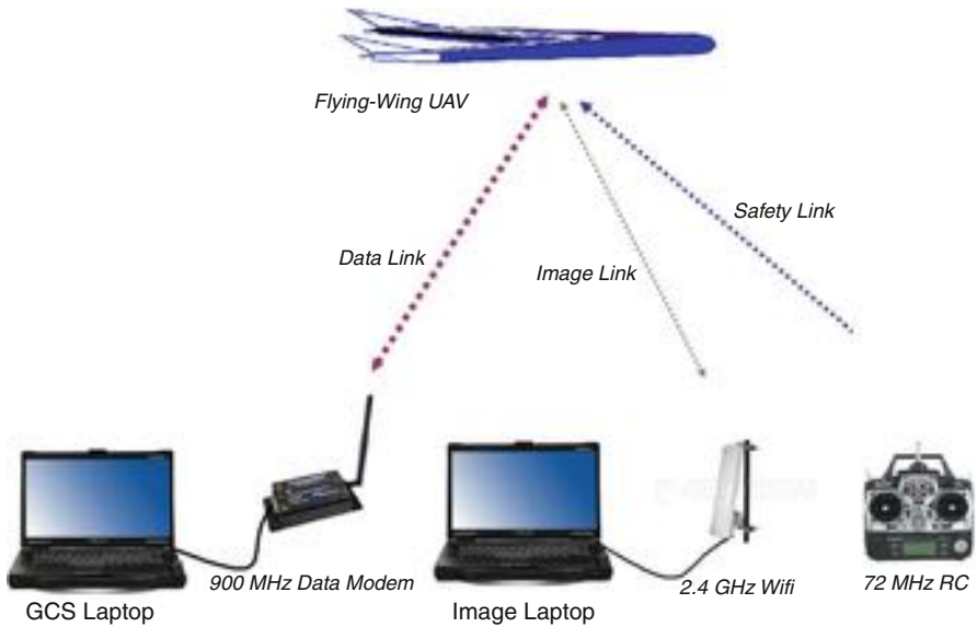
Fig. 117.7 AggieAir SUAS system diagram (Haiyang Chao 2009)
