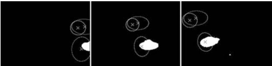
Fig. 112.11 Heliv receives the information of the alarms detected by Marvin and fuses this information with the information obtained using its infrared camera. This figure shows the estimated position and uncertainty of the alarms detected by Marvin projected on the Heliv's infrared camera
