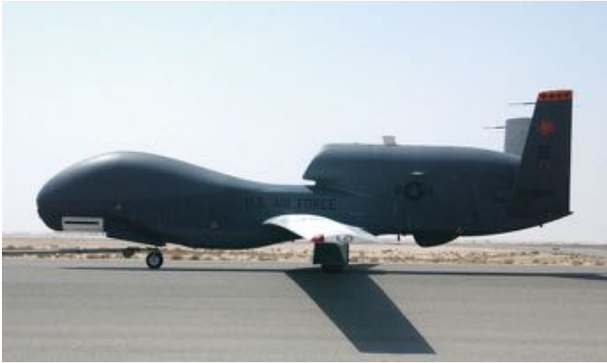
Fig. 4.17 The RQ-4 Global Hawk is a high-altitude, long-endurance UAV. It was the first UAV to do a transpacific crossing (Newcome 2004) (Photo Credit: US Air Force, Master Sgt. Jason Tudor)
