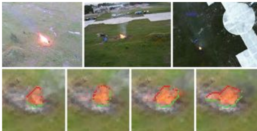
Fig. 112.19 Top: left, image from Heliv, after stabilization and feature extraction; middle, image from Marvin after stabilization and feature extraction; right, image from Karma. Bottom: details of the extracted contours. Green: fire front. Red: top of the flames
