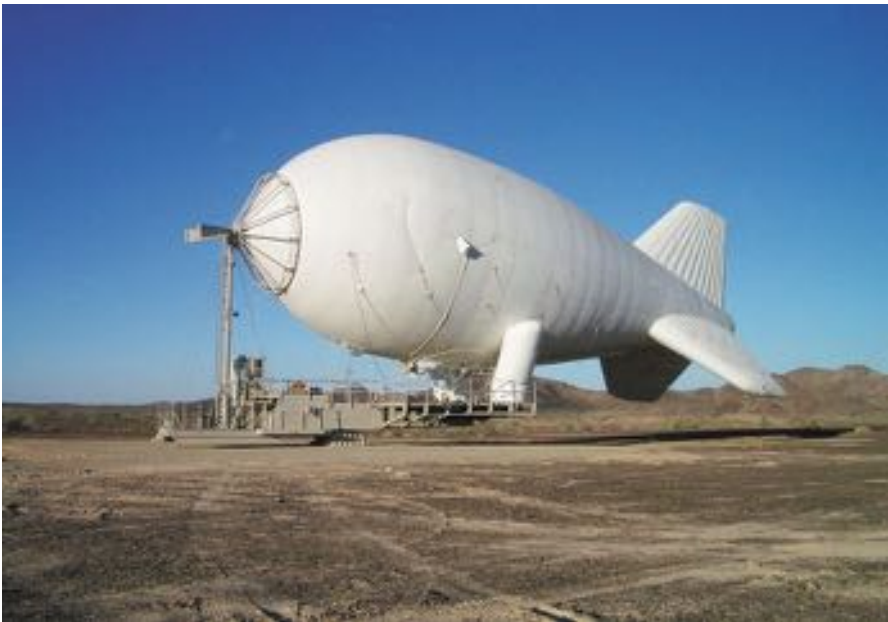
Fig. 4.31 The Persistent Threat Detection System (PTDS) is equipped with a high-resolution EO/IR payload used for surveillance (Photo Credit: US Army)
