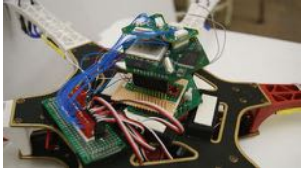
Fig. 12.16 Onboard electronics of Dexterous Hexrotor
