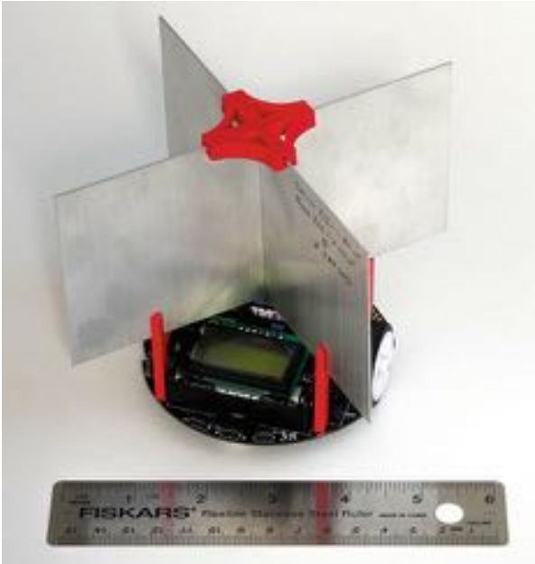
Fig. 79.17 Line following RADAR target (with 6'' (15 cm) size reference)
