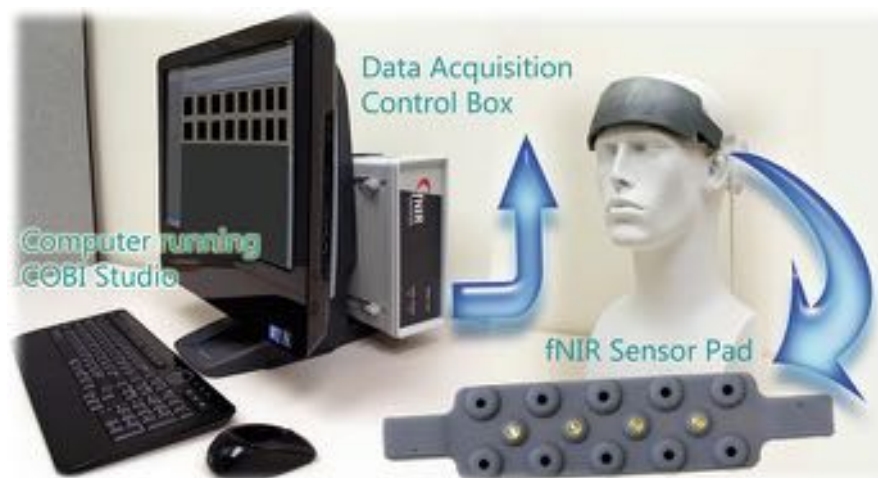
Fig. 102.2 Overview of the CW fNIR system. Flexible sensor housing four LED light sources, ten photodetectors and wires. Computer running COBI Studio collects data through hardware control box
