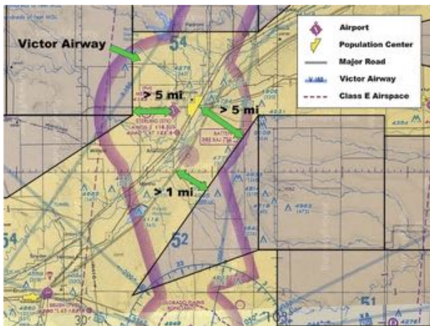
Fig. 90.4 Considerations for the sizing, shape and location of each polygon , with green arrows indicating minimum distances and obstacles including 5 miles or more from both airports and built-up areas, 1 mile from major highways, and consideration for Victor airways, which the FAA does not allow loitering in
