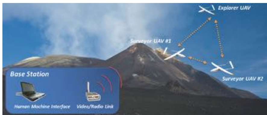
Fig. 111.4 A graphical representation of the interaction between three cooperating UAVs flying in the proximity of a crater
