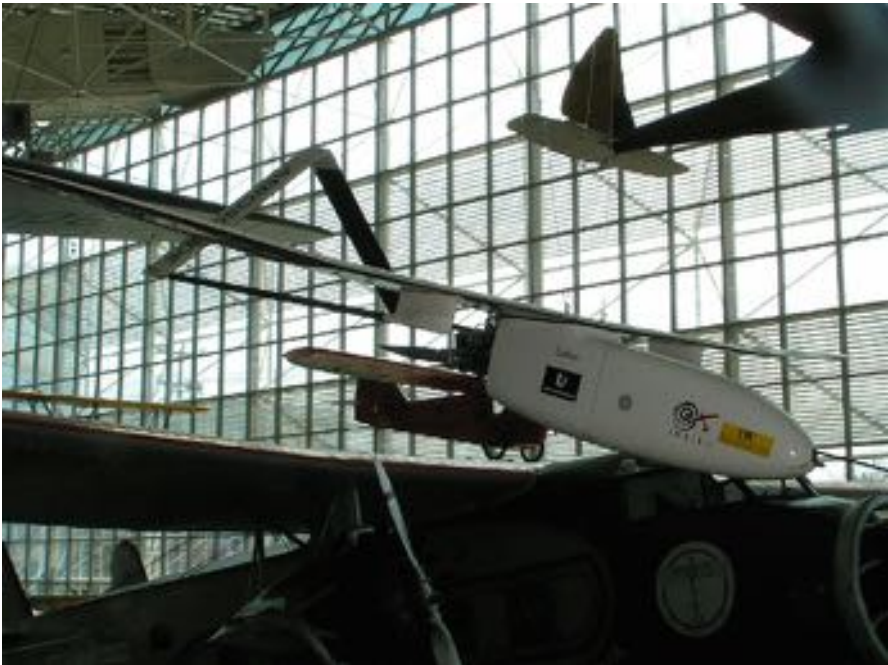
Fig. 4.24 The Aerosonde Laima was the first UAV to make a transatlantic crossing (Newcome 2004) (Public domain photo)
