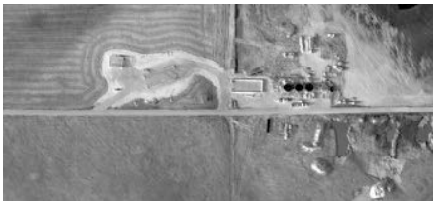
Fig. 117.2 A 10 cm-resolution mosaic of thermal imagery collected by the AggieAir™ small unmanned aerial vehicle system (Coopmans et al. 2012 )
