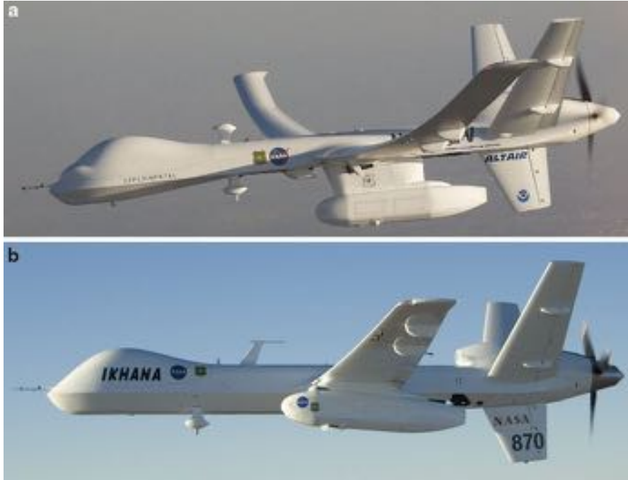
Fig. 113.17 (a & b) (top) The NASA Altair UAS (modified Predator-B) platform in flight during 2006 Western States UAS Fire Imaging Mission Series. The AMS sensor was carried in the pod mounted below the fuselage. (bottom) The NASA Ikhana UAS (Predator-B) platform in flight during the 2007 Western States UAS Fire Imaging Mission Series. The AMS sensor was carried in the pod mounted under the wing (Images courtesy of NASA)
