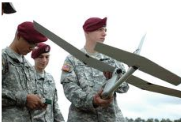
Fig. 4.27 The Raven is a backpackable UAV for “over the hill” and route reconnaissance that evolved from the Pointer UAV. In the photo paratroopers are training with an RQ-11 Raven (Photo Credit: US Army, Sgt. Amanda Jackson)
