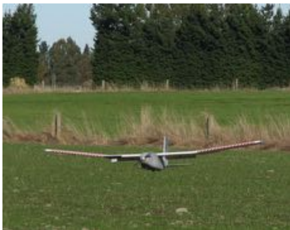
Fig. 95.4 AggieAir PRS UA with high-visibility reflective markers
