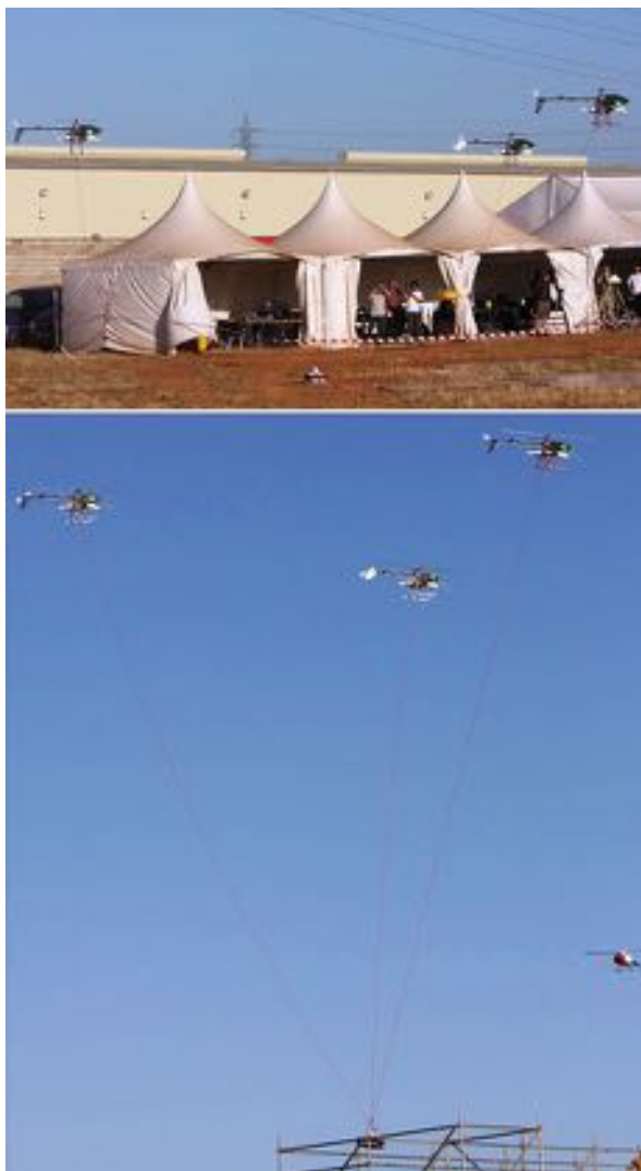
Fig. 114.19 Three UAVs transporting a pan-tilt wireless camera to the roof of a building with a height of 12 m in Utrera (Spain) in May 2009. The images show the mission during the take-off ( top picture ) and shortly before ( bottom picture ) the load deployment. On two pictures, a fourth helicopter is visible, which was used to acquire airborne video footage of the mission
