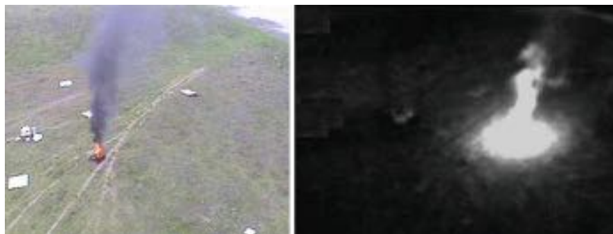
Fig. 112.3 (Left) Visual image taken in one multi-UAS fire perception experiment. (Right) Infrared images of the same scene taken with one Raytheon 2000AS OEM infrared micro-camera
