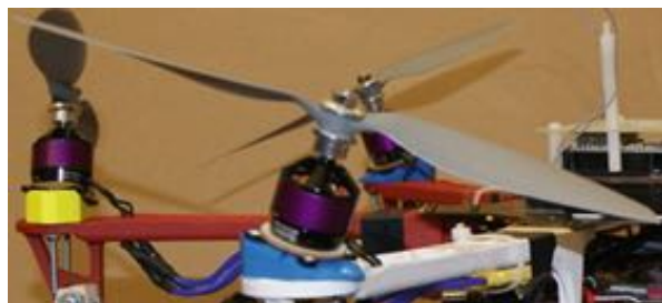
Fig. 12.15 Motor mounted on a 20° ABS plastic adapter
