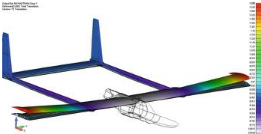
Fig. 8.17 Simulated deflections caused by in-flight loads
