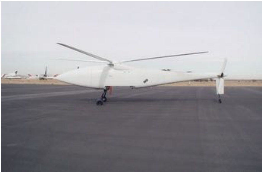
Fig. 4.22 The A-160 Hummingbird built by Boeing/Frontier. It is a demonstrator for improvements in range endurance and controllability (US Department of Defense Office of the Secretary of Defense 2005 ) (Photo Credit: US DoD)
