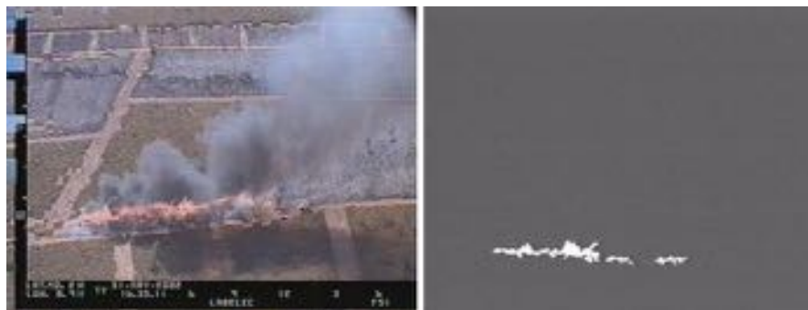
Fig. 112.15 Images from UAS onboard visual ( left ) and infrared ( right ) cameras taken during a fire monitoring experiment
