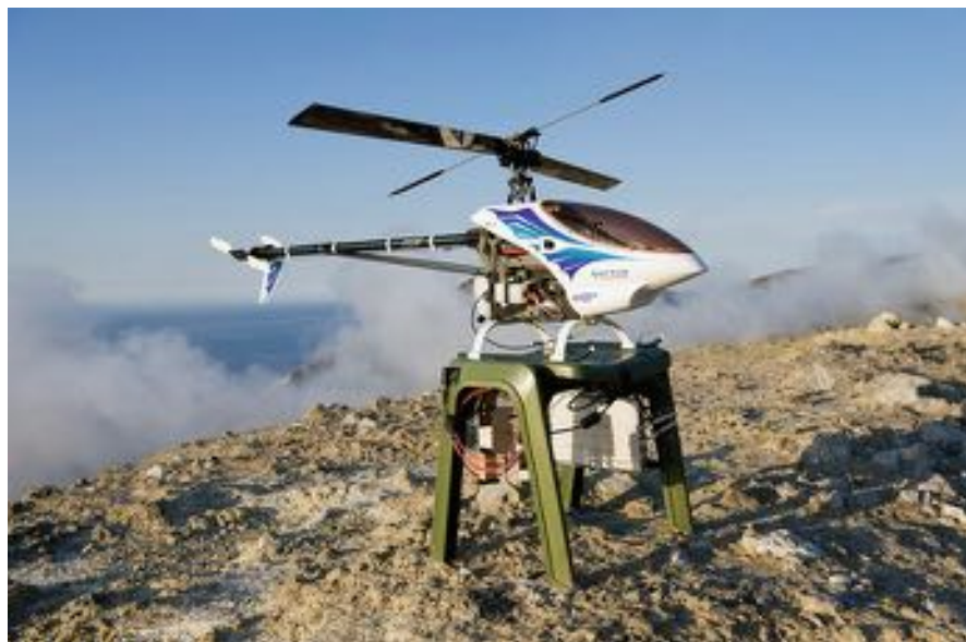
Fig. 111.8 The Thunder Tiger Raptor 90 helicopter and the sensor payload used to measure volcanic carbon dioxide fluxes (Photo: ©Rolex Awards/Marc Latzel)
