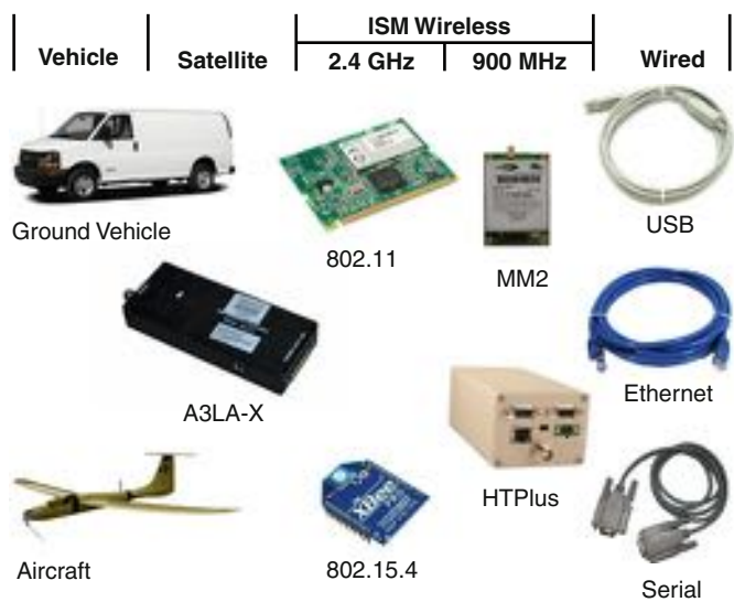
Fig. 34.2 The various transport methods supported by the network-centric architecture and resulting software
