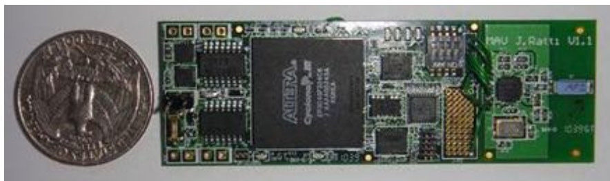
Fig. 57.20 MARC-2 (Cyclone III, TI 55xx DSP) dual core
