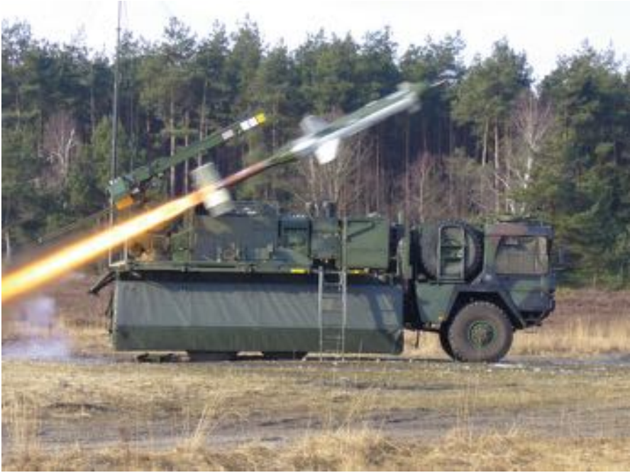
Fig. 4.13 German reconnaissance drone CL-289 (Photo Credit: Karsten Franke)
