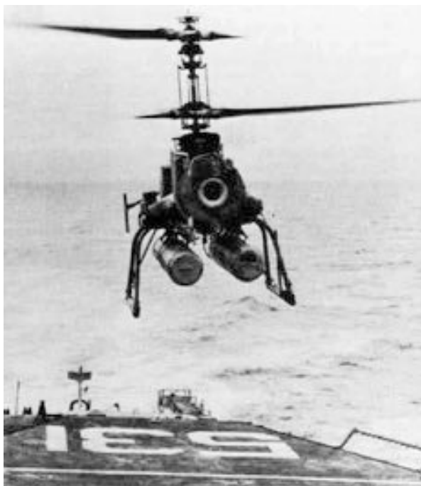
Fig. 4.9 A QH-50 DASH-drone armed with torpedoes over the flight deck of the USS Hazelwood (Photo Credit: US Navy)
