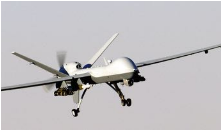
Fig. 4.18 The MQ-9 Reaper is an updated version of the Predator UAV. It is primarily used as a persistent hunter-killer UAV for critical time-sensitive targets and secondarily for intelligence gathering (US Department of Defense Office of the Secretary of Defense 2007) (Photo Credit: US Air Force, Staff Sgt. Brian Ferguson)
