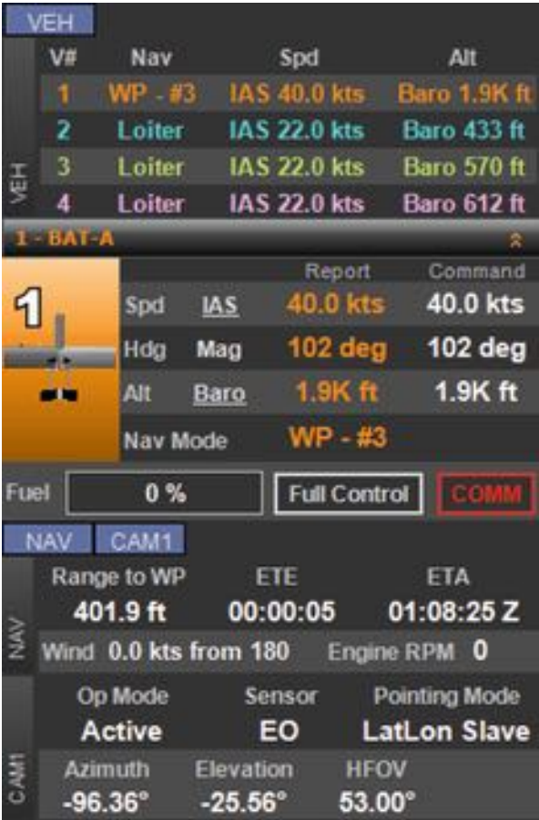
Fig. 101.2 Sample vehicle alert and summary tool from Vigilant Spirit Control Station
