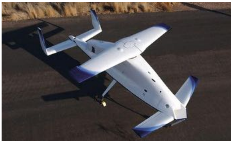
Fig. 4.37 The X-50 aircraft built by Boeing Corp. It is a technology demonstrator for the Canard Rotor Wing (CRW) configuration which combines hovering capabilities with high cruise speeds (US Department of Defense Office of the Secretary of Defense 2005 ) (Photo Credit: US DoD)
