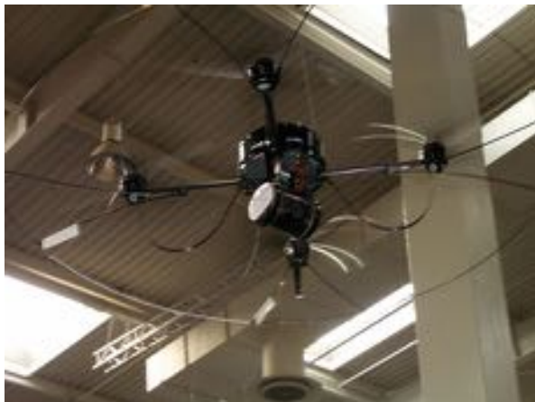
Fig. 4.38 The AirRobot AR 100-B features autonomous landing when it is out of range or when the battery is low (Public domain photo)
