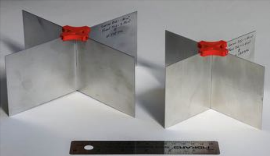
Fig. 79.14 Quad-dihedral RADAR reflectors (with 6'' (15 cm) size reference)
