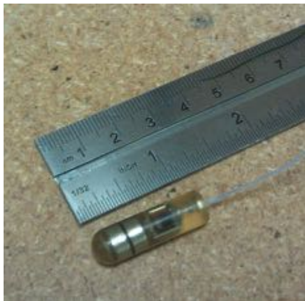
Fig. 117.16 Implantable radiotransponder tags, allowing remote detection of fish of various sizes (From Lotek corporation (2012))
