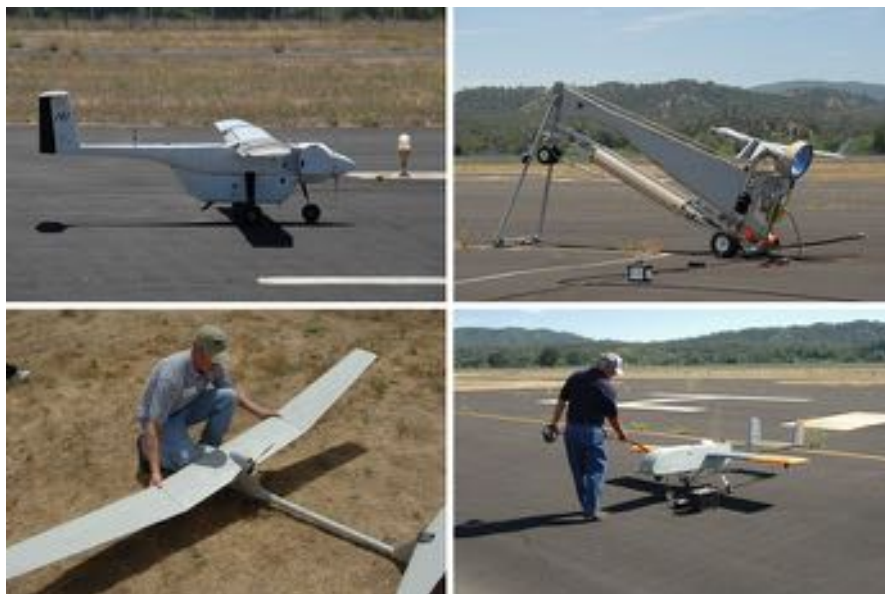
Fig. 113.16 UAS in June 2006 USFS/NASA Fire Imaging Demonstration, Ft. Hunter Liggett, CA ( Upper left ) APV-3 UAS used as an over-the-horizon communications relay platform; ( upper right ) In Situ (Boeing) A-20 ScanEagle on catapult launch assembly; ( lower left ) AeroVironment Puma, hand-launched UAS; and ( lower right ) IntelliTech Vector-P UAS, in preflight tarmac test
