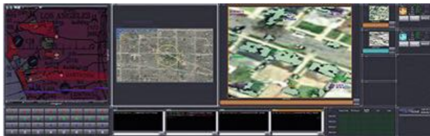
Fig. 101.17 Alternate Vigilant Spirit Control Station layout with both large and small video windows
