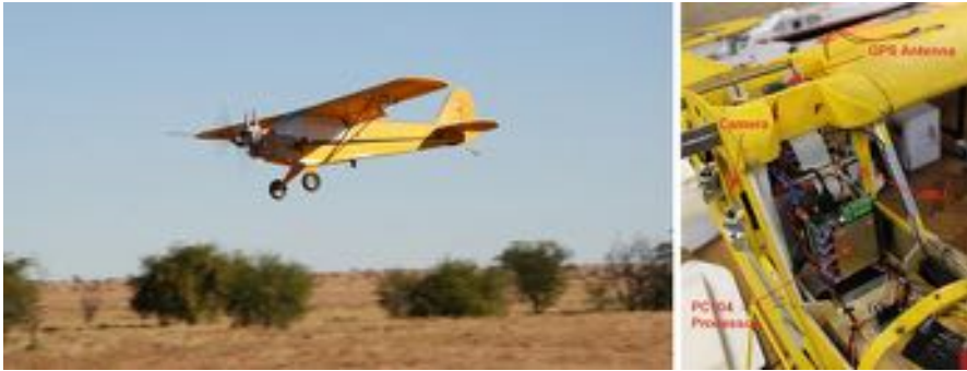
Fig. 22.4 UAV and localization sensor payload system: left , the J3 Cub, a small UAV used primarily for airborne photographic mapping; right , the sensor payload box carried onboard the UAV consisting of a triaxial IMU, GPS receiver, and PC104 computer stack for logging and processing data
