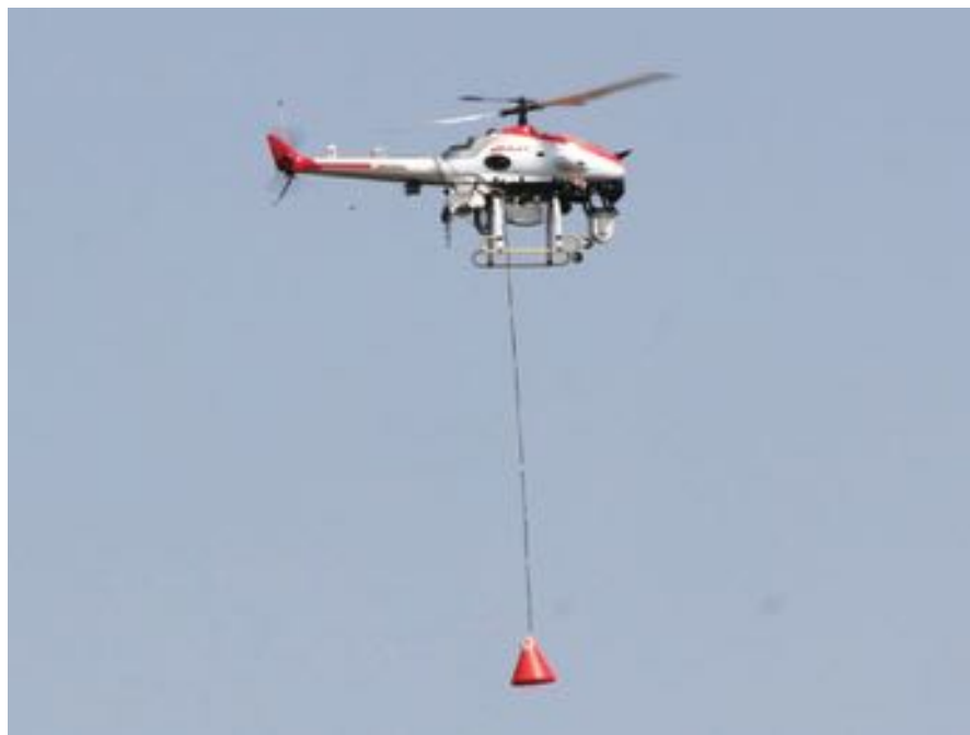
Fig. 111.17 The YAMAHA Motor Co. Ltd. RMAX-G1 helicopter carrying the cesium magnetometer, attached by means of a rope (Copyright © 2011 Taylor & Francis Group)
