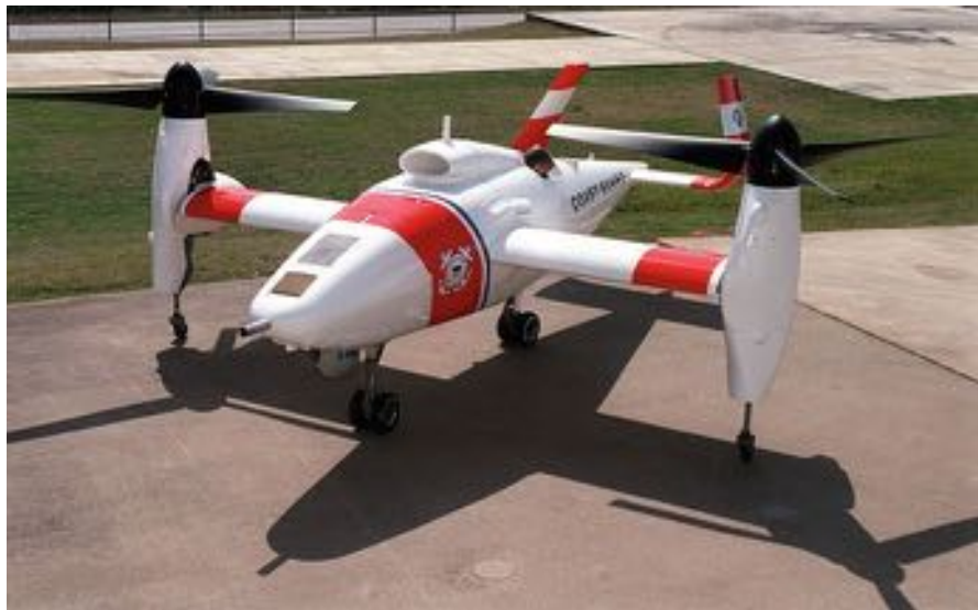
Fig. 4.36 The Eagle Eye is a tilt-rotor UAV developed by Bell Helicopter. It was selected by the US Coast Guard for its Deepwater program but was put on hold in 2007 (Photo Credit: US Coast Guard)
