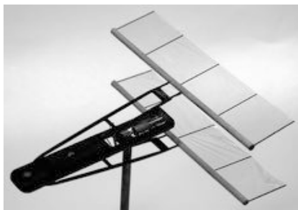
Fig. 56.16 MAV-sized biplane propulsion test model
