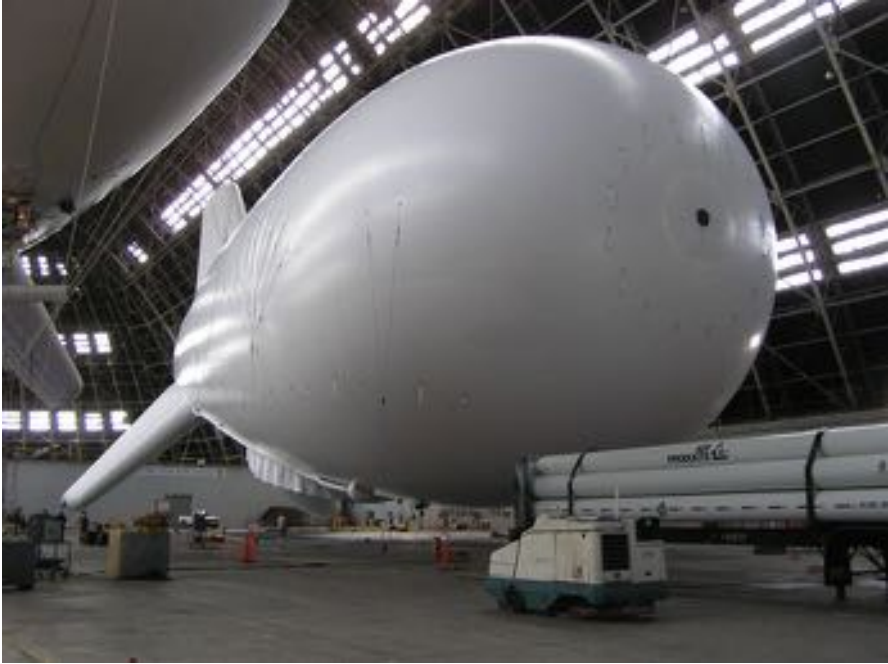
Fig. 4.30 Joint Land Attack Elevated Netted Sensor (JLENS) by Raytheon/TCOM capable of providing over-the-horizon surveillance (Photo Credit: US Army)
