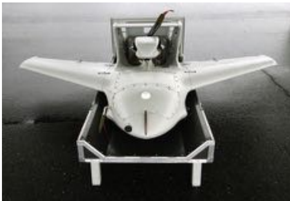
Fig. 4.19 The Neptune, a reconnaissance UAV capable of water landings (Photo Credit: US Navy)
