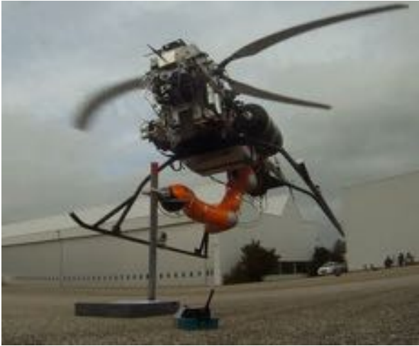
Fig. 114.4 Experimental setup for precision control with integrated vision system. This is the first worldwide setup in outdoors involving an autonomous helicopter equipped with a robotic arm for manipulation
