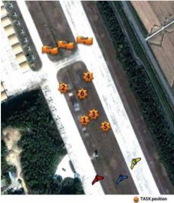
Fig. 63.20 Task-assignment scenario for three UAVs with a no-fly zone
