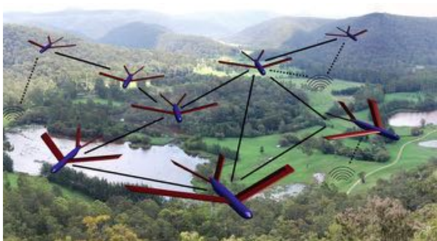
Fig. 82.1 A UAV swarming concept where only a subset of the UAVs are directly controlled by human operators. These operators influence the remaining UAVs through an interaction network between vehicles
