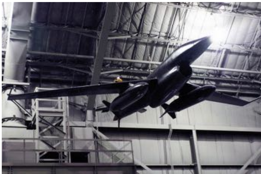
Fig. 4.7 The AQM-34Q, one of several variations of the Ryan Model 147 unmanned reconnaissance drone, used in the 1960s and 1970s (Photo Credit: National Museum of the USAF)
