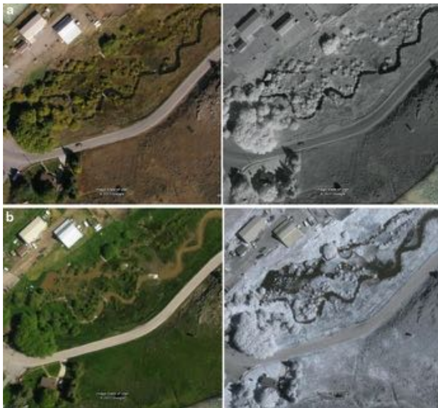
Fig. 117.12 Multispectral data collected from an agricultural scene: (a) Visible and NIR data before flood. (b) Visible and NIR data after flood
