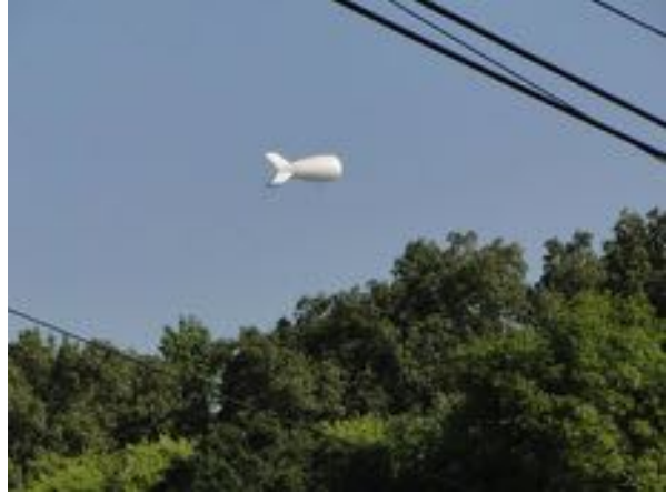
Fig. 4.32 The Rapid Aerostat Initial Deployment (RAID) is a smaller version of the JLENS, used in missions of area surveillance and force protection against small arms, mortar, and rocket attacks (Photo Credit: US Army)
