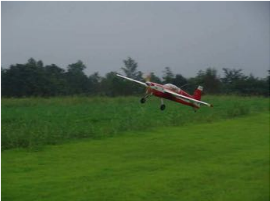
Fig. 29.4 The GTEdge aircraft with a high (greater than 1) thrust-to-weight ratio
