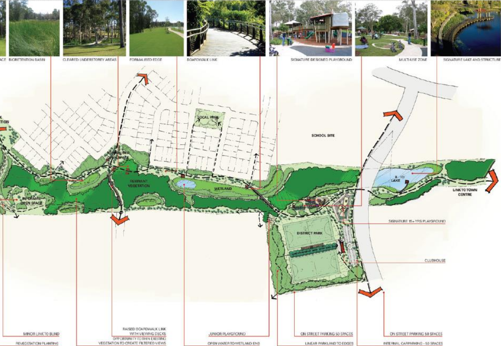
Figure 21 — Multiple use open space corridor incorporating WSUD BMPs, a constructed wetland and bioretention systems to treat stormwater runoff from adjoining development areas.
