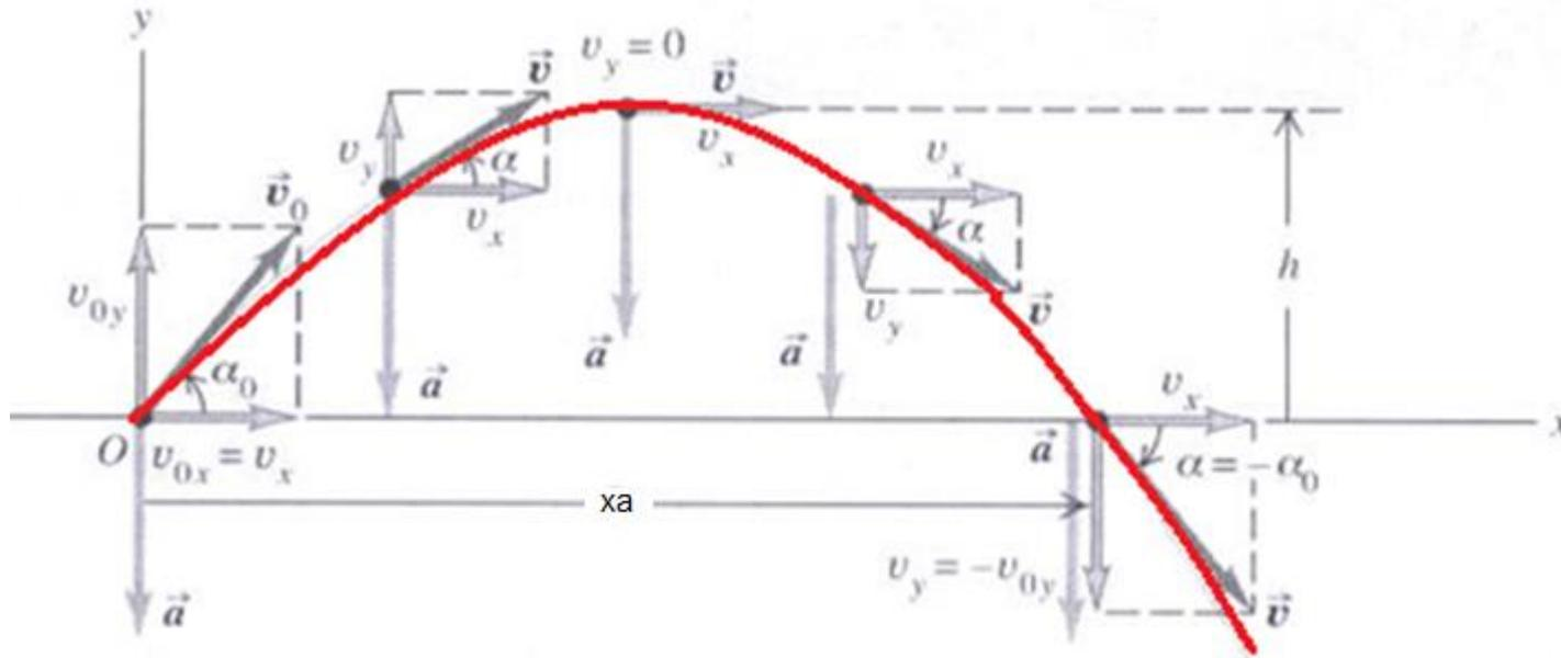
$$x_0 = 0; \quad y_0 = 0; \quad v_{0x} = v_0 \cos(\alpha_0); \quad v_{0y} = v_0 \text{sen}(\alpha_0)$$
