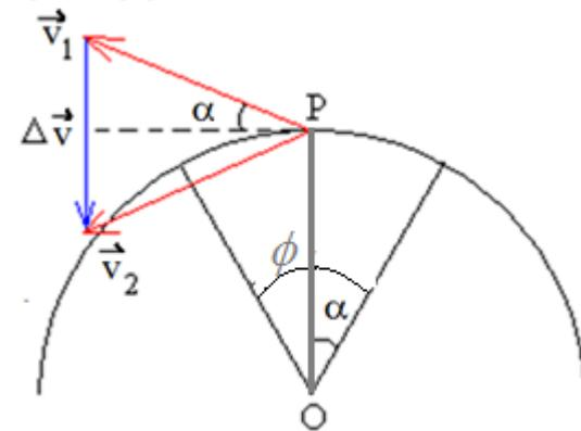
$$\therefore a_{\text{média}} = \frac{(\Delta v)_n}{\Delta t} = \frac{2 \times v \times \text{sen}(\alpha)}{\frac{2 \times r \times \alpha}{v}} = \frac{v^2}{r} \times \frac{\text{sen}(\alpha)}{\alpha}$$
