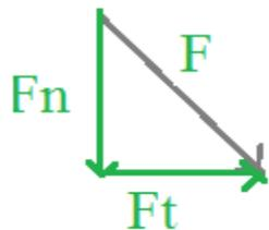
$$\begin{aligned} F_n &= F \sin(45^\circ) \\ F_t &= F \cos(45^\circ) \end{aligned}$$
