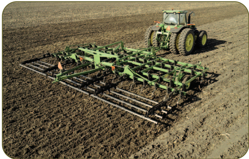
FIELD CULTIVATOR--W/ COILED TINE HARROW ATTACHMENT
