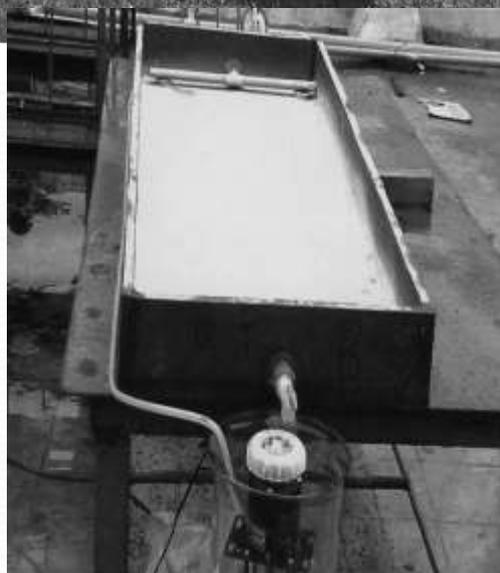
TiO<sub>2</sub> TFFBR. Size: 144 cm×52 cm×10 cm; solution flow rate: 750 ml min<sup>-1</sup>; batch size: 5 l.
