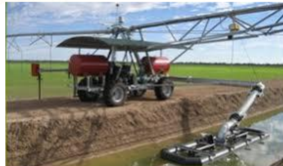
Fig. 1.39. Travel lateral irrigating on one side of the supply canal
