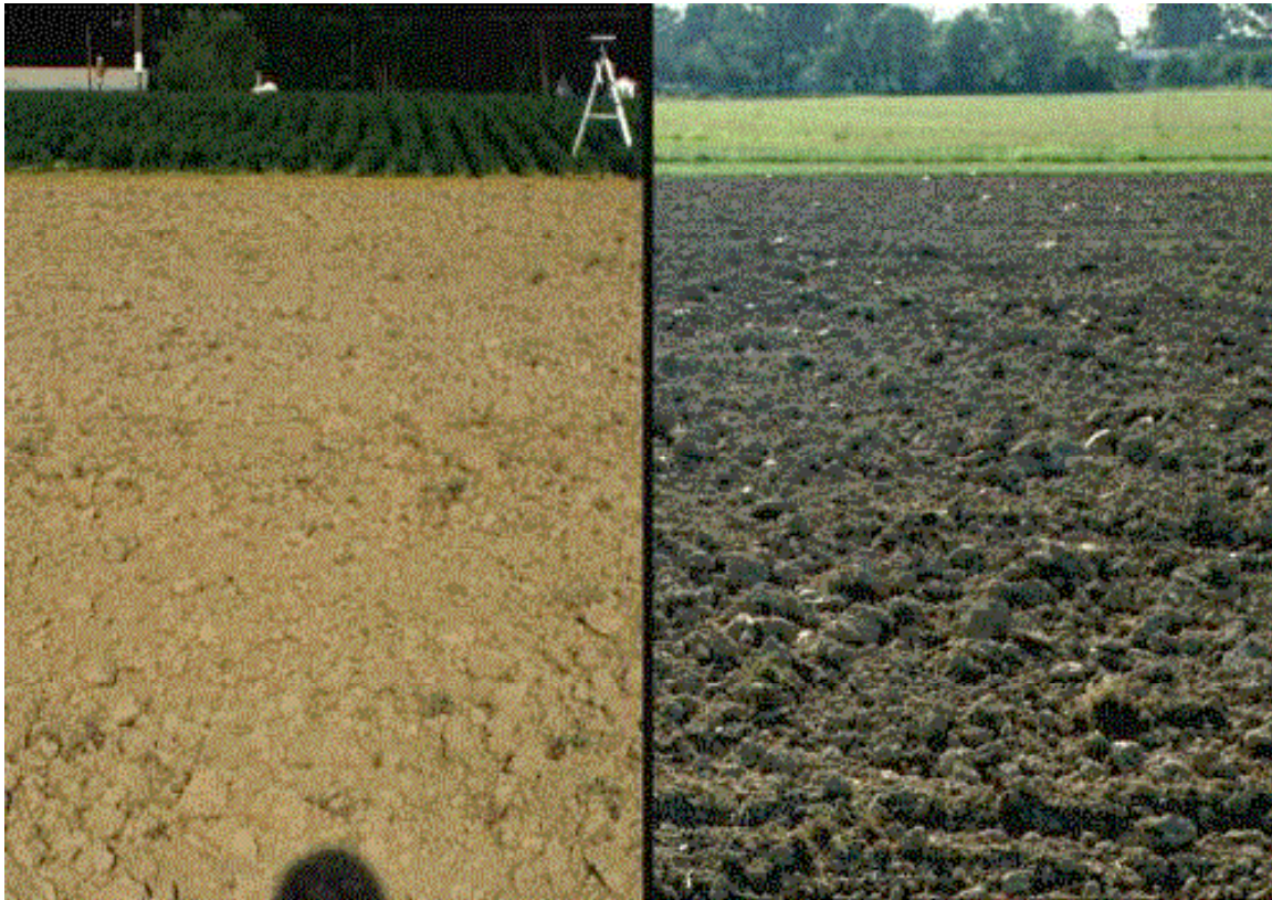
Figure 3.15. Viewing a bare soil field at a constant view and sun zenith angles, but opposite azimuthal angles, i.e, 180° apart.
