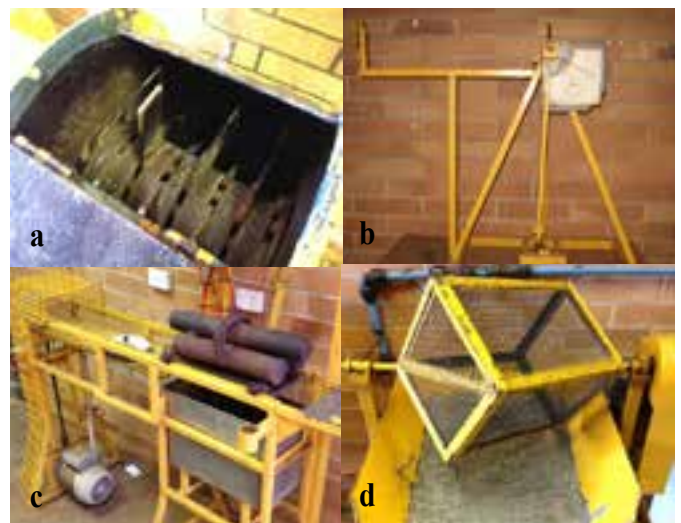
Figure 3. Equipment used to measure fibre quality components; a) hammer mill for cane preparation, b) impact resistance, c) shear strength and d) short fibre content.
