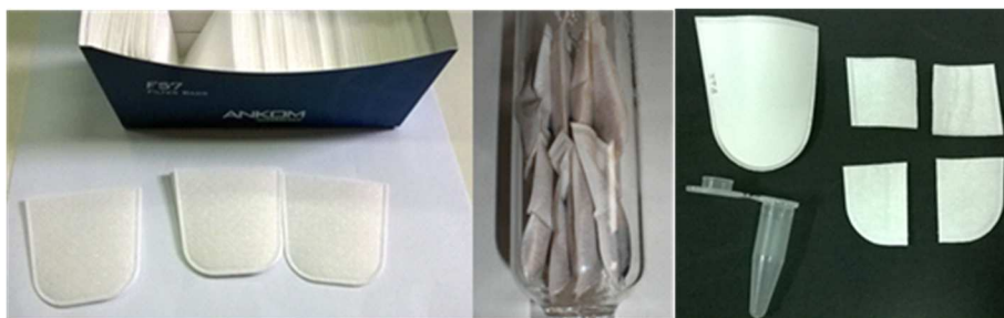
Figure 2.1 F57 filter bags (Ankon), Soxhlet extractor with 8 samples ready for extraction, and a filter bag sized to fit 4 samples.
