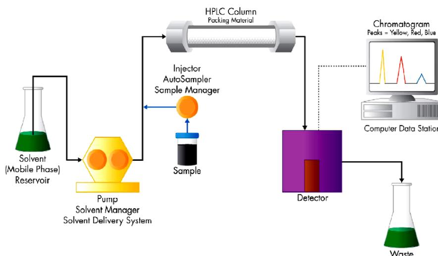
**Figure 10:** schematic diagram of High-Performance Liquid Chromatography (HPLC) system (from Water corporation, 2012)
